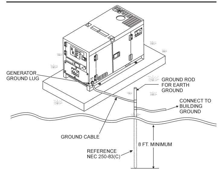
Figure 2. Typical Generator Grounding Application
